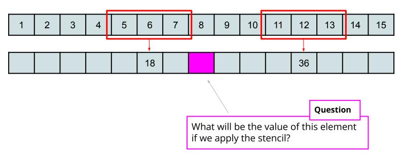
Lets understand how shared memory works by trying to apply a **1-D stencil** to a 1-D array!
