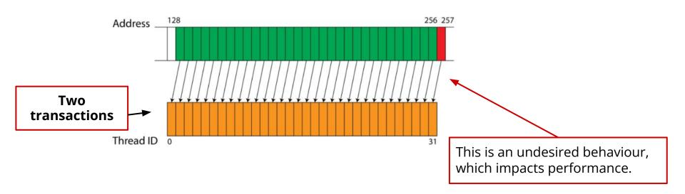
If the data accessed by the threads in a warp are not in the same burst section, the data access will take twice as long
