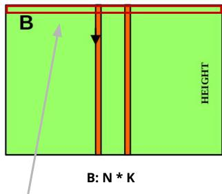
**First iteration** → a warp of 32 threads reads element 0 of the first 32 columns
